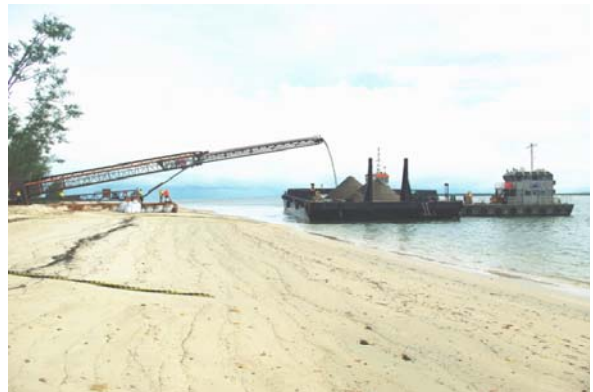
Loading Barge with concentrate to be taken to off-shore ship
