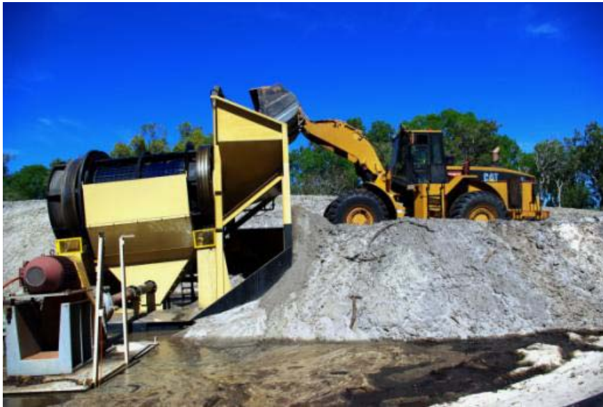
Front End Loader feeding ore into In-Pit Screening / Slurry unit
